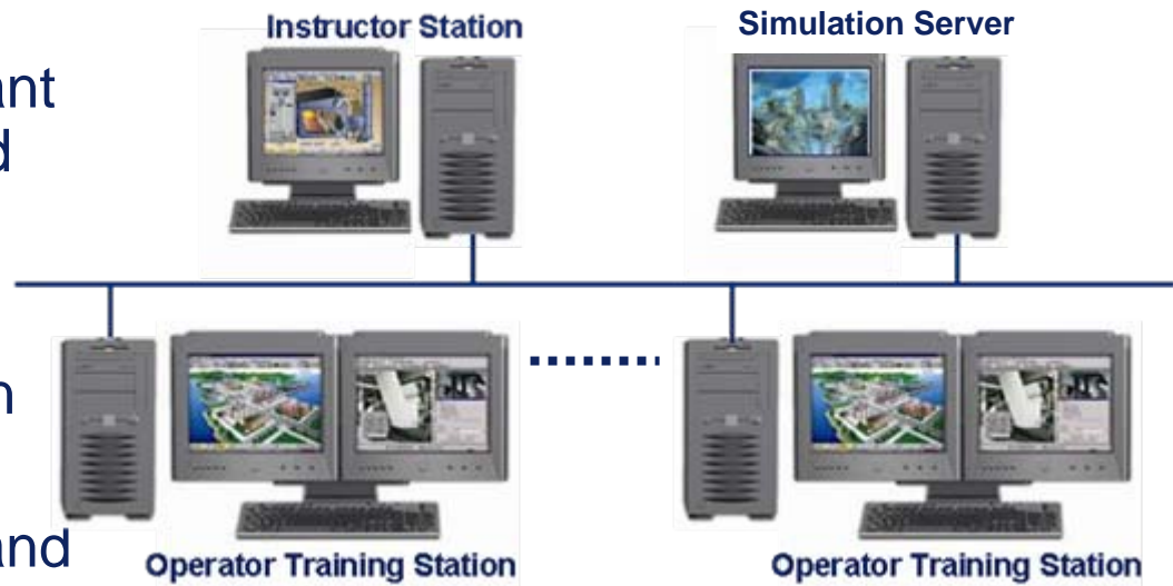
DeltaV OTS example architecture
