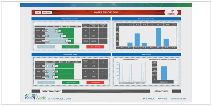
PKN Orlen uses real-time dashboards to monitor the impact of water and wastewater operations on the environment and to control deviations from acceptable operating limits.
