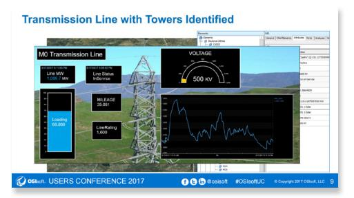
**Transmission tower visualization:** The combination of geo-registered data, images, and PI System sensor data is visualized in PI Coresight to enable predictive analytics and maintenance strategies.
